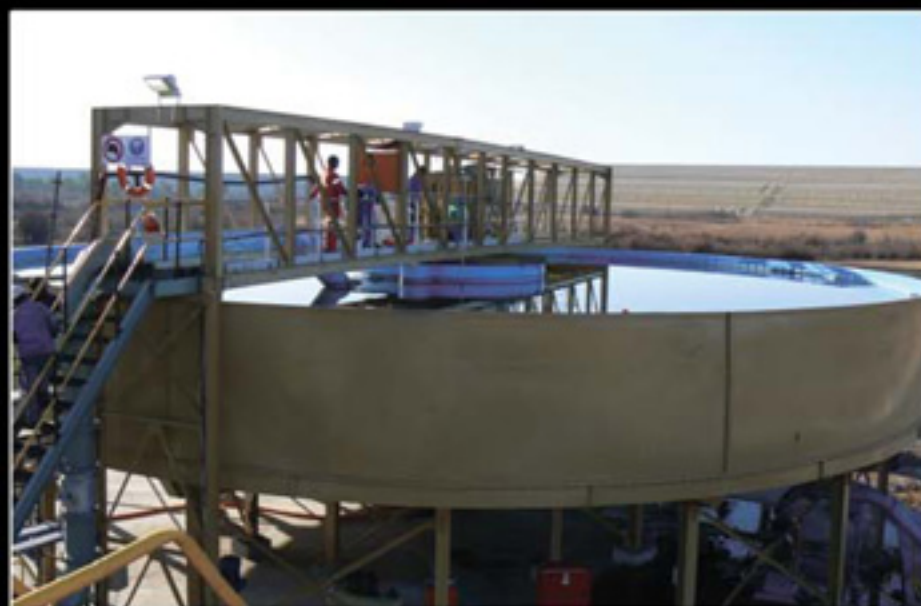
21m \phi thickener from bolted construction
