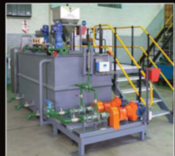
MIP-200 Flocculant Plant
